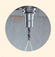
• Coolant-Thru Capabilities: Jet Coolant Splash with J-Type Nut
