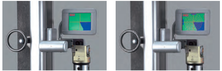
Display of angular grid (1 degree increment) for inspection of Tool cutting edge
