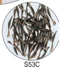
Material:S53C V=500m/min. f=0.25mm/tooth S=10000min -1 F=10000mm/min.
