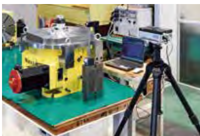
Indexing Accuracy Measurement by Laser
