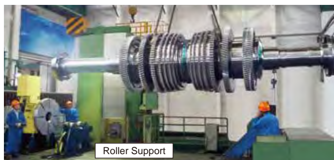
CNC1201 Indexing of the turbine shaft. Turbine shaft is supported and clamped by the roller support.
