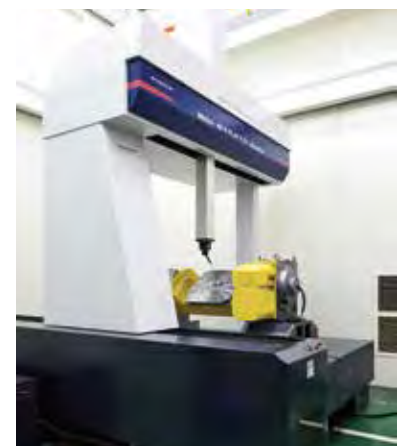
Accuracy measurement with large 3 Dimensional Measuring Machine
